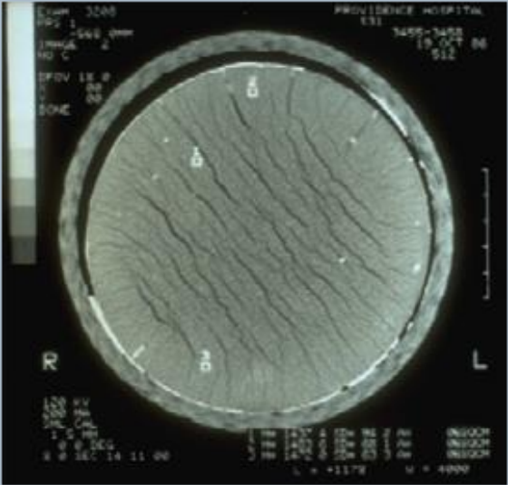
Longitudinal Fracturing (no lifting support – cradle)
